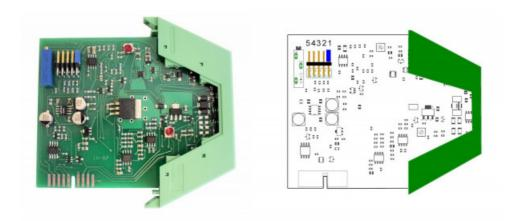
The input sensitivity can be adjusted by moving the jumper. The input sensitivity for position 1 is indicated in the type designation. In position 5, the amplification can be set in a continuously variable manner using trimmer "TR".
