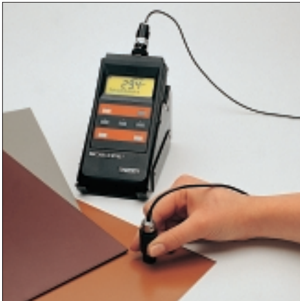
DELTASCOPE® MP10 displays individual measurement values without statistics, it has no serial interface (no printing, no data transfer) and does not store measurement values.
