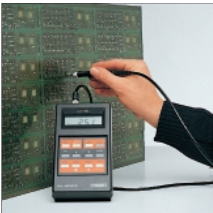
The CU-SCOPE CMP1A is used to measure copper plating thickness in PCB through holes.
