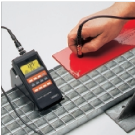
Measurement of a duplex coating (paint/zinc coating on iron) using EDX10 probe and DUALSCOPE® MP40.
