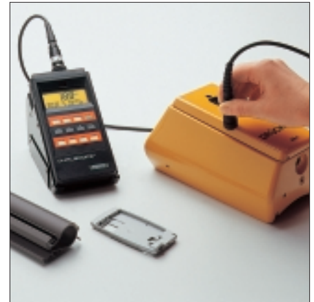
Measurement of the paint coating thickness on a curved surface using ETD3.3 probe and DUALSCOPE® MP40.
