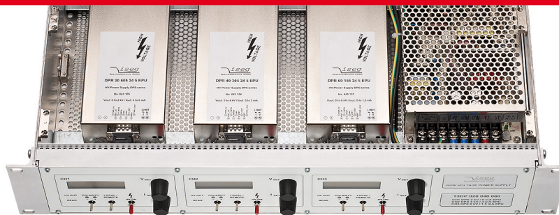
© iseq Spezialelektronik GmbH 19" THQ device equipped with three DPS high voltage modules
