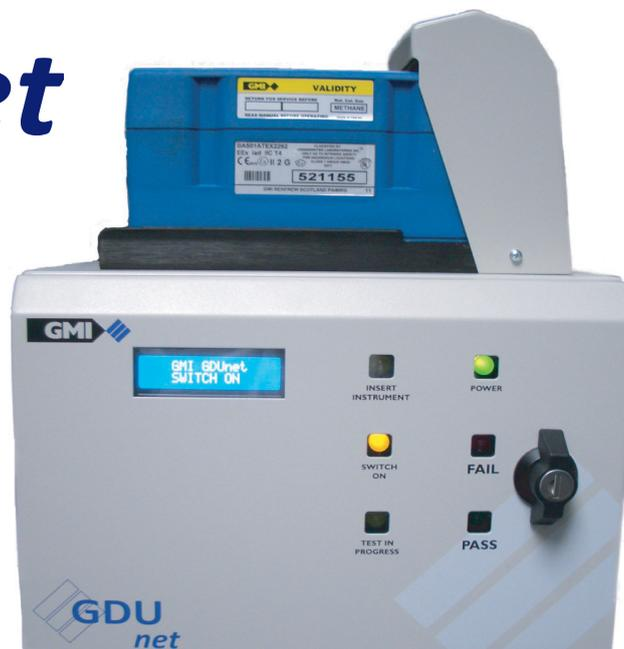
The GDU*net* automates the essential task of regular instrument bump testing and calibration, ensuring that the Gasurveyor family of instruments are functioning correctly. This Gas Delivery Unit has 3 modes of operation, for all user requirements:
