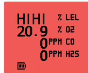
Red display in alarm conditions
