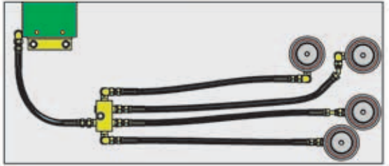
Four U.4600 gas springs linked using DADCO's Y-400 hose, fittings and a Common Control Panel.
