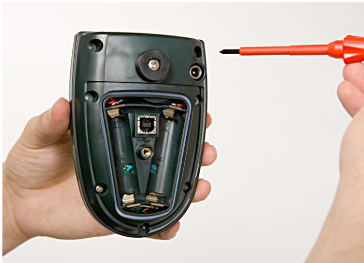
Figure 16- Remove the sensor cap screws
