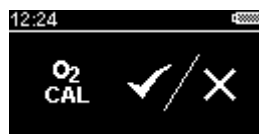
Figure 12 - Oxygen fresh air calibration confirmation screen
