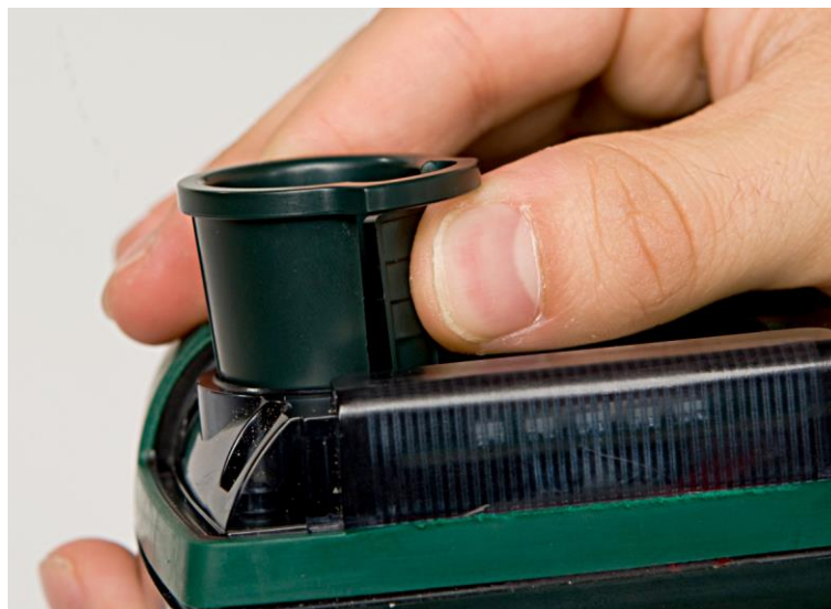
Figure 21 - Squeeze the extraction tool
