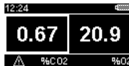
Figure 5 - The main gas display showing that carbon dioxide levels have triggered an alarm
