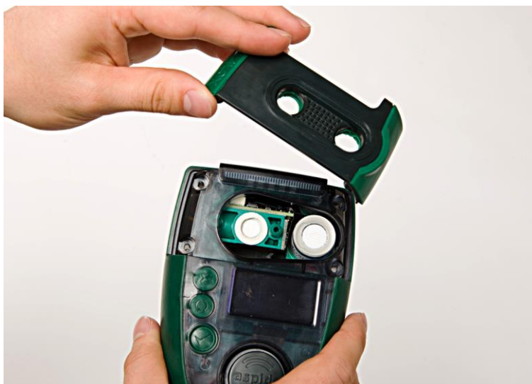
Figure 17 - Remove the sensor cap
