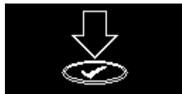
Figure 6 - Display shown when the man-down alarm is triggered
