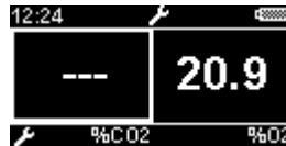
Figure 11 - Display showing a carbon dioxide sensor fault
