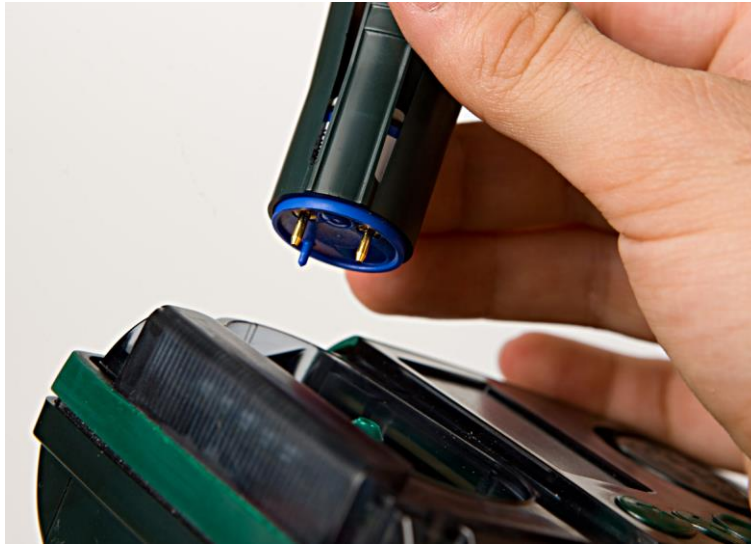
Figure 22 - Removing the oxygen sensor
