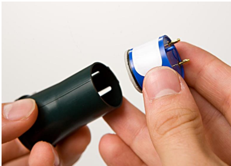
Figure 23 - Insert the new sensor into the extraction tool
