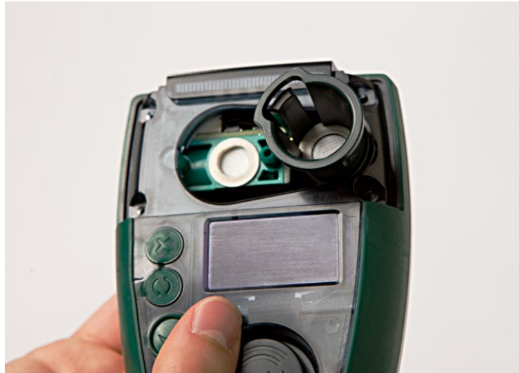
Figure 20 - Correct extraction tool position
