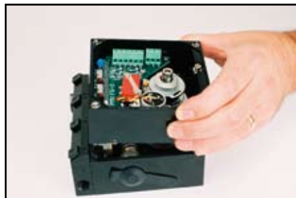
Place F5 unit on top, tighten screws
