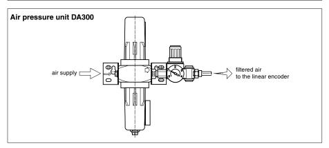
For applications where the Linear Encoders are used in harsh environments (e.g. oil and coolants), there are two methods of extra protection beyond the enclosed unit's standard set of sealing lips.
