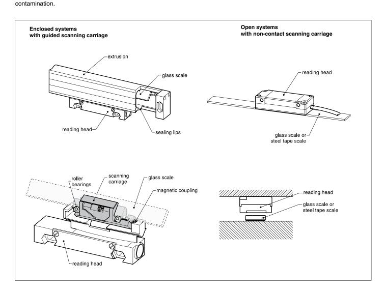
Enclosed Linear Encoders have a roller bearing, self-guided scanning carriage. The scanning carriage is spring loaded to track properly within the encoder head mounting tolerance range. A set of rare earth magnets couple the scanning carriage to the mounting base of the encoder head.
