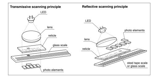
The scale consists of a glass carrier and reflection-type phase grating. The scanning reticle acts as transmission phase grating.
