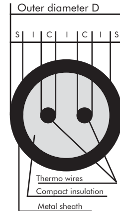
Cross-section of sheathed cable
