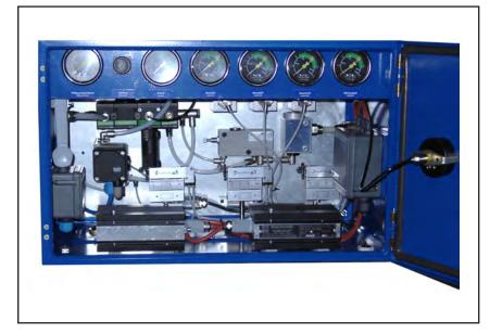
Special version of the MANOCOMB ® pressure switch as the maximum pressure limiter with pneumatic switch contacts for safety valve control devices.
