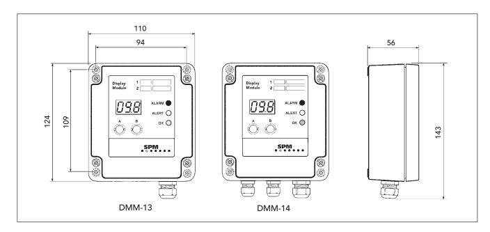
DMM-13 and DMM-14 are condition display modules for 4-20 mA analog signals. Measured quantities and ranges are selected from a preprogrammed list (13 programs) or from user defined programs (7 programs). DMM-14 has two extra cable inlets of type Pg7.
