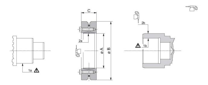
Only if the shrink disc is removed and then remounted must its conical surfaces as well as the shank and underneath of the screws' heads be cleaned and greased using a grease containing high pressure additives (MoS2).
