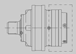
If a negative brake is used, measure the temperature on the body of the brake, by its disks.
