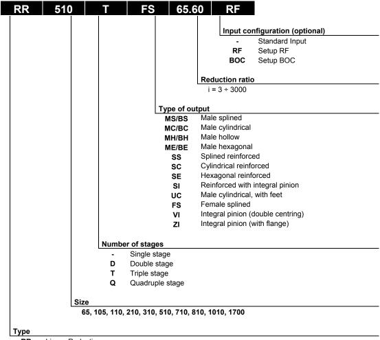
RR Linear Reduction gearRA Angular Reduction gear
