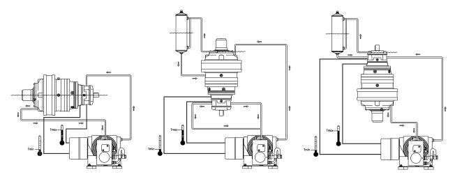
The size of the delivery pipes must take into account the distance between the cooling unit and the reduction gear, being careful not to exceed an overall line pressure drop of 2-3 bar in the operating temperature range ( $30^{\circ}\text{C} \div 90^{\circ}\text{C}$ ).
