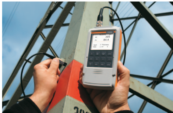
DUALSCOPE® FMP40 using the duplex probe FDX13H
