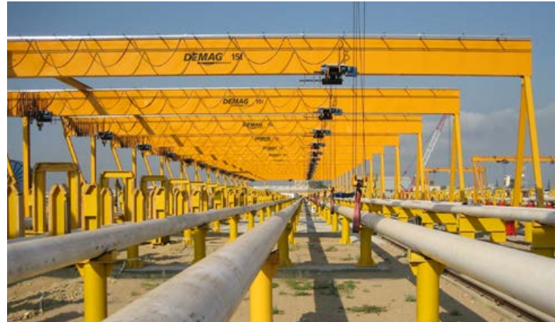
DH hoist units operating outdoors in high temperatures in a pipeline construction application
