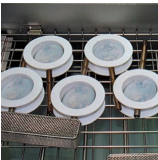
Decontamination by ultrasonic cleaning
