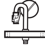
Bottom Plate, Float, Needle and Seat Assembly Part No. 52200000 For Models 506-507, 926-927 Top Load
