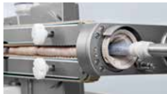
↑ Casing spooling with holding device and linking nozzle
