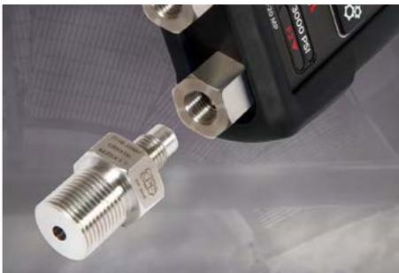
**CPF** Crystal Pressure Fittings<sup>♦</sup> are machined in high-strength 316 Stainless Steel to operate at 10 000 psi/700 bar. Removable CPF adapters shift everyday thread wear away from the HPC50 Series' ports, while a self-venting weep hole alerts you before you disconnect from a pressurized system.
