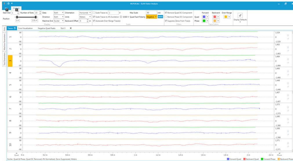
Test traces display of either or both Quad and Phase on all traces.
