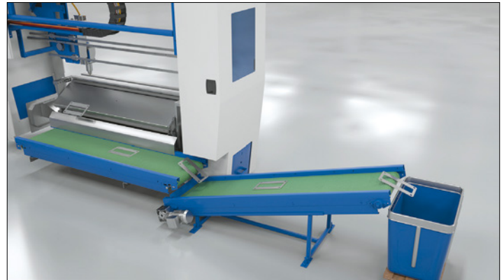
Additional conveyor to unloading point
