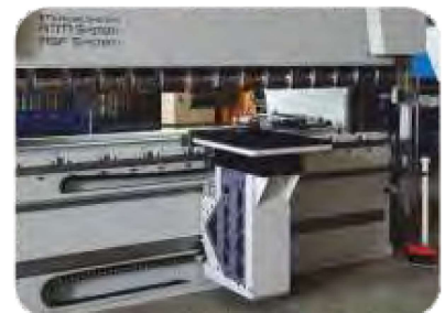
Innovative CNC Bending Aid with automatic height adjustment
