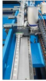
Servo geared motor with precision rack and pinion drive.
