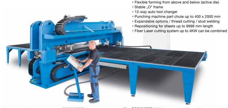
The new CNC punching machine **BOSCHERT 4020** completes the proven MultiPunch series and is specially designed for the processing of sheets in the so-called super format of 2.000 x 4.000 millimeters. With its universal punching head, the 4020 enables the user a flexibility and double-sided forming of sheet metal up to a sheet thickness of 6 mm. Up to 28 tons of punching force are available. for this. The newly developed O-frame gives it the necessary stability.
