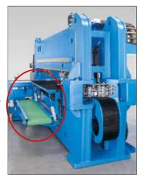
welded steel construction guarantees the highest stability for punching sheets up to 12,7 mm thickness. Part chute on the left up to part size 400 x 2000 mm. A conveyor belt move the parts to the operator side.
