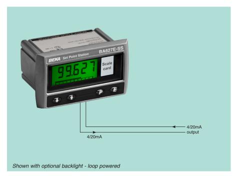
The BA627E-SS set point station enables the current flowing in a 4/20mA loop to be manually adjusted from within a process area via the front panel push buttons. Housed in a rugged stainless steel enclosure with a toughened glass window the BA627E-SS is ideal for installations in harsh industrial and marine environments and where the front of the instrument is likely to be impacted.
