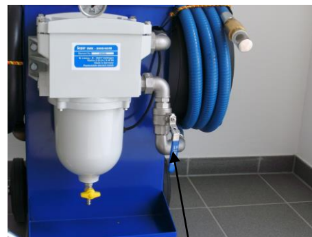
Shut-off valve opened
