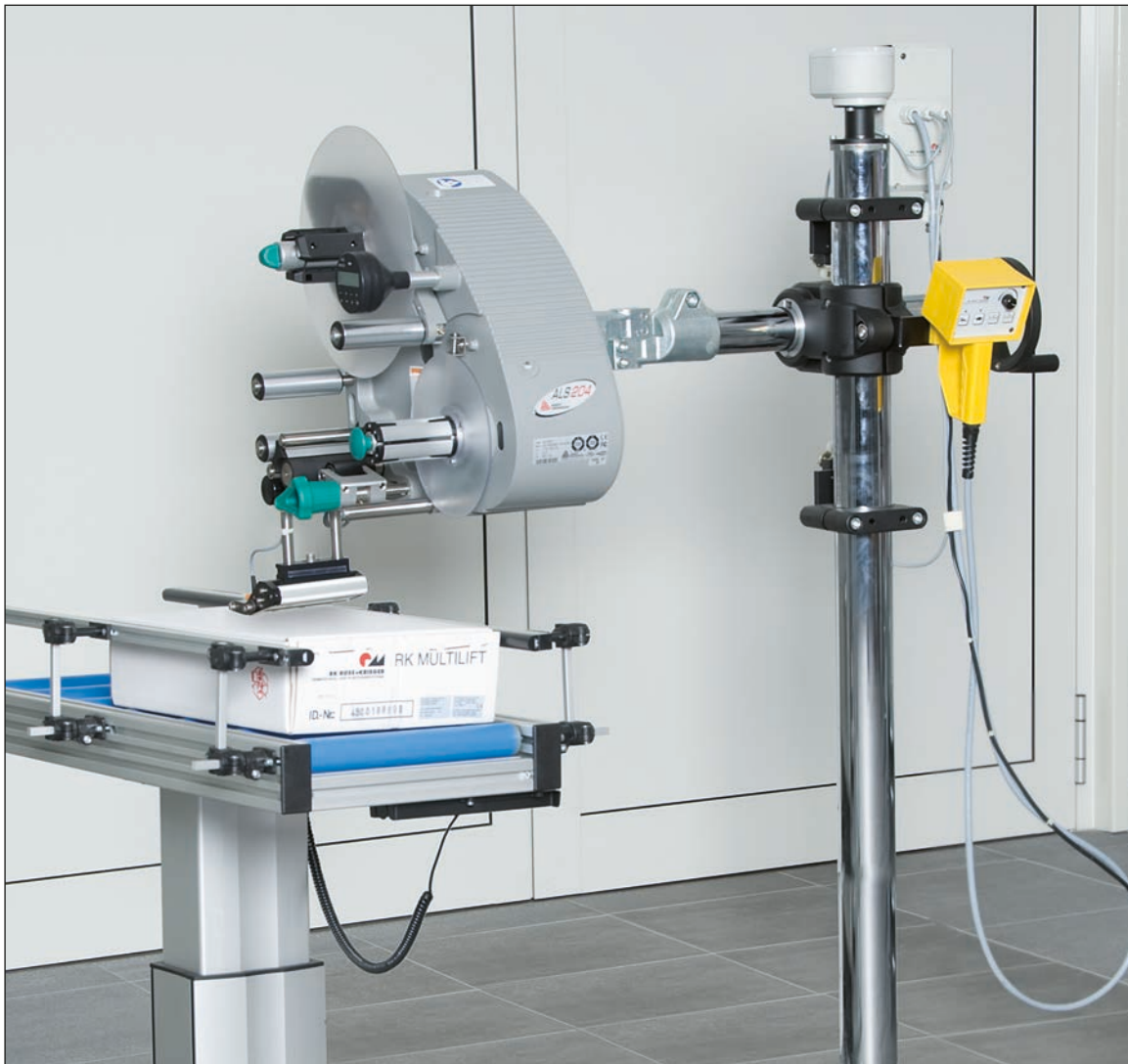
Positioning of a labelling machine via a crossing E tubular linear unit
