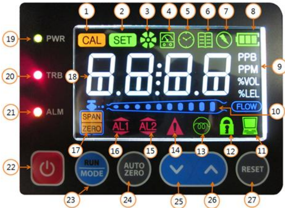
[Figure 3. Front panel display part]
