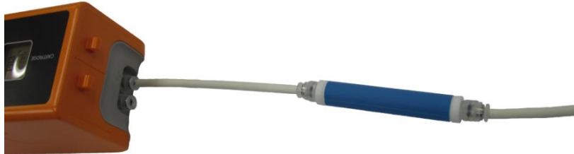
Figure 4. Sampling Port Connection
