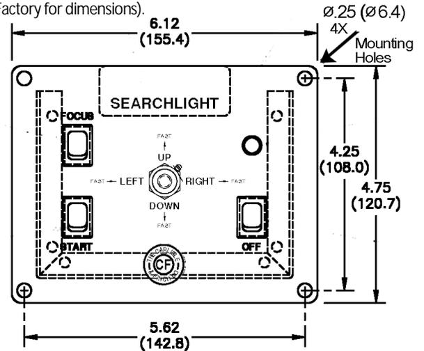
C4-2-1 Master Station.....Depth = 6.5in (166mm)
