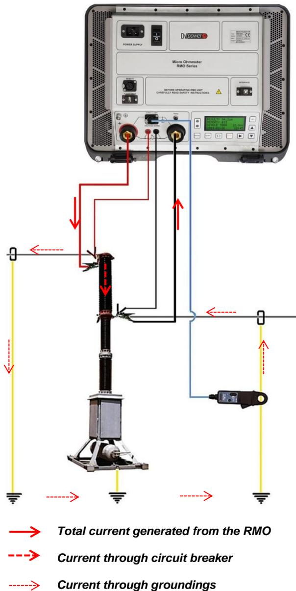
Using the RMO-C with a current clamp-meter is an additional safety feature. Measurement of a circuit breaker contact resistance is done with both sides of the breaker grounded. The RMO-C device will measure the current through the ground circuit connection and add this value to the selected test current value to provide the selected test current through the test object.
