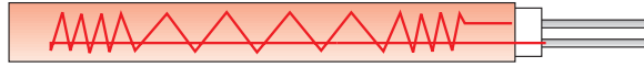
Anfang und/oder Ende stärker beheizt Reinforced power distribution on one or both ends
