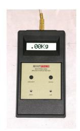
BINTPRES M50 Brush Force Meter can be equipped with both SM5 or SM5/F probes, depending on application.
