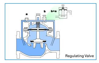
The 2-way control device provides sensitive, accurate, and constant modulating, control of the main valve. The main valve does not fully open, as the control device prevents total draining of the control chamber.
