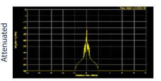
Power levels of each signal can be adjusted with resolution finer than 0.1 dB.
