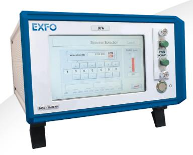
The XFA is electronically controlled and wavelength tuning ranges from 1450 nm to 1650 nm. The bandwidth is factory-set and can be selected at purchase between 50 pm and 800 pm with respect to the center wavelength.
