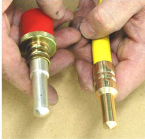
Figure 7 – Guide Tube Removal and Fixed End Stops
