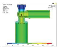
Reduces thermal stress, improves thermal cycling and increases the lifetime of the valve.
