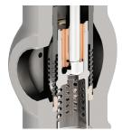
Suitable for installations where erosion caused by wet steam, or where high velocities can have an adverse effect on seat leakage tightness. The distribution of pressure drops in this configuration reduces the steam velocity across the sealing surfaces.
