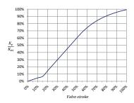
Allows for greater rangeability and flow control at lower flow rates. The graph shows how at the first ~15% of the stroke, the change in flow coefficient increases by only 5%.
