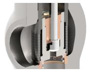
Provides a leakage tightness according to ANSI FCI 70-2 / EN 1349 Class V. The pilot plug lowers the pressure drop across the plug, which reduces the required actuating forces and allows smaller actuators to be used.
