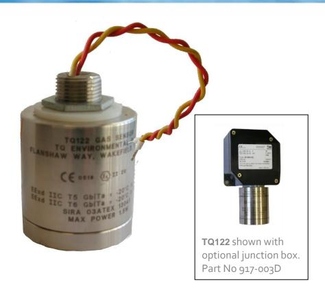
The **TQ122** series is a range of flameproof (Ex d) toxic gas and Oxygen deficiency sensors for use in zone 1 and zone 2 hazardous areas. The **TQ122** sensors are configured as 2-wire 4-20mA transducers for interface with the TQ4000 or TQ8000 control panel series or Third Party control systems.
