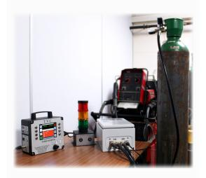
The GPM features a 5.7-inch LCD screen for a clear view of the monitored Oxygen level. The Oxygen level can be set by the user to be displayed in percent (%) or parts per million (ppm). The Zirconia sensor can measure Oxygen levels from 5% down to 0.0001% (5000 to 1ppm). Data logging of the Oxygen level and operation time is directly onto a 4GB pen stick flash drive and can be programmed by the user to record at preset intervals.
