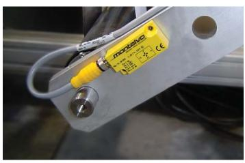
Montalvo DPS-1 mounted to a dancer arm running a foil that requires quick and accurate feedback.
