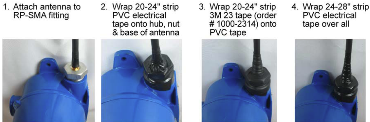
Figure 2-7: Water Proofing Antenna Connections
