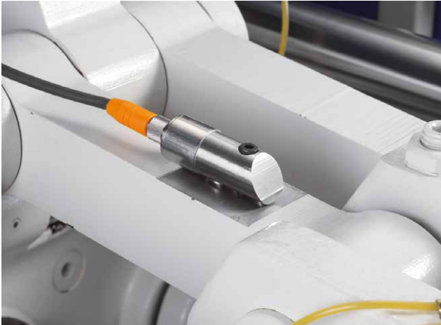
Fig. 8: Indirect force measurement on knuckle joint
