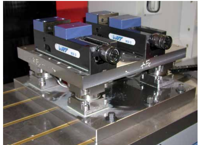
Fig. 1: Exemplary application of a 3-component force transducer, here using the Types 9347C/9348C as an example
