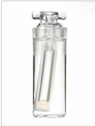
Figure 4: Zero calibration chamber (MR-Ch 0-calibration). The zero solution is outside the silicone tubing and pure water is inside. The oxygen in the water inside the tubing diffuses through the silicone tubing into the zero solution where it is consumed.
