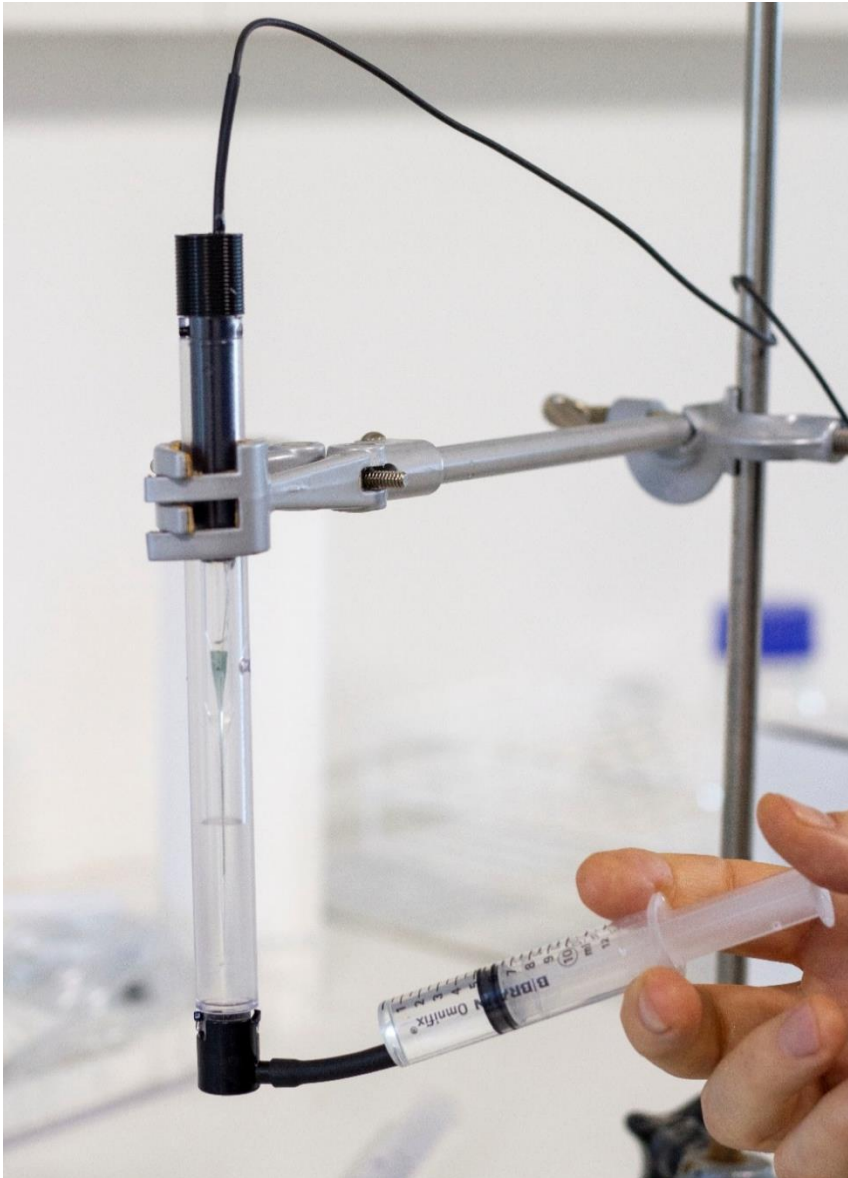
Figure 2:Oxygen microsensor with the calibration cap mounted. Calibration solution is injected with the 10 ml syringe.
