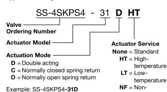
For dual-mounted assemblies (two valves mounted to one actuator), insert **DM** into the ordering number. Example: SS-4SKPS4-31D**DM**HT
