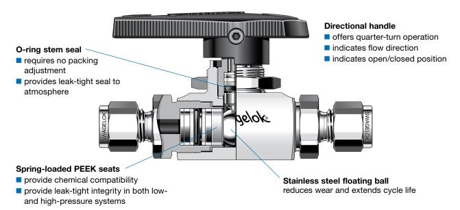
Swagelok® SK series ball valves offer low-torque, quarterturn operation in a compact design providing positive shutoff in applications up to 6000 psig (413 bar). Other features include:
