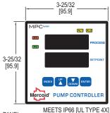
The **Series MPC JR Pump Controller** provides versatile level control in a standard 1/4 DIN package. Designed for use with almost any style level transmitter the unit displays the present level and main set point value. Incorporated in the MPC JR is programmable level differential for on/off control of one or two pumps, valves, or other devices through two SPDT relays.
