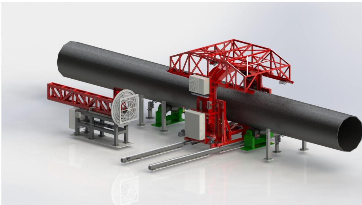
Figure 5.1. Device measuring the diameter and roundness while testing the pipe
