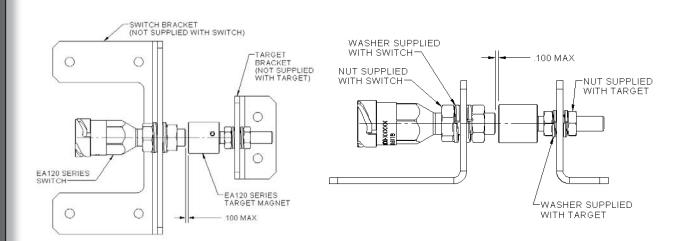
Figure reflects switch in "actuated" position. Two 5/8-18 jam nuts and two 5/8" lock washers supplied with switch. Target magnet EA120-10001 required for operation (sold separately). Average hysteresis: 0.20" (5mm) to 0.40" (10mm)
