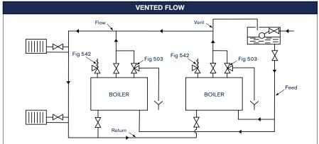
In both types of installation, there must be no isolating valve fitted between the Fig 503 and the boiler, vent pipe or drain.
