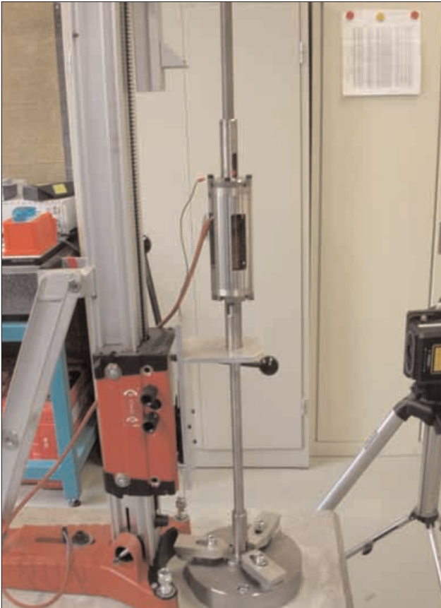
Figure 8: Symmetrical pulse generator vertical arrangement. Both sides are coupled to steel bars for two sided impulse extraction. Notice the slits in casing and mounting flanges steel for getting optical access for the LDA-measurements.
