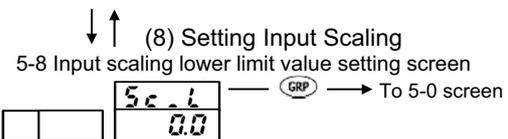
A lower limit value of scaling for linear input (mV, V, mA) is set. During sensor input, the lower limit of measuring range is displayed and no change is possible. A set value is unable to be changed during RUN in the PROG mode.
