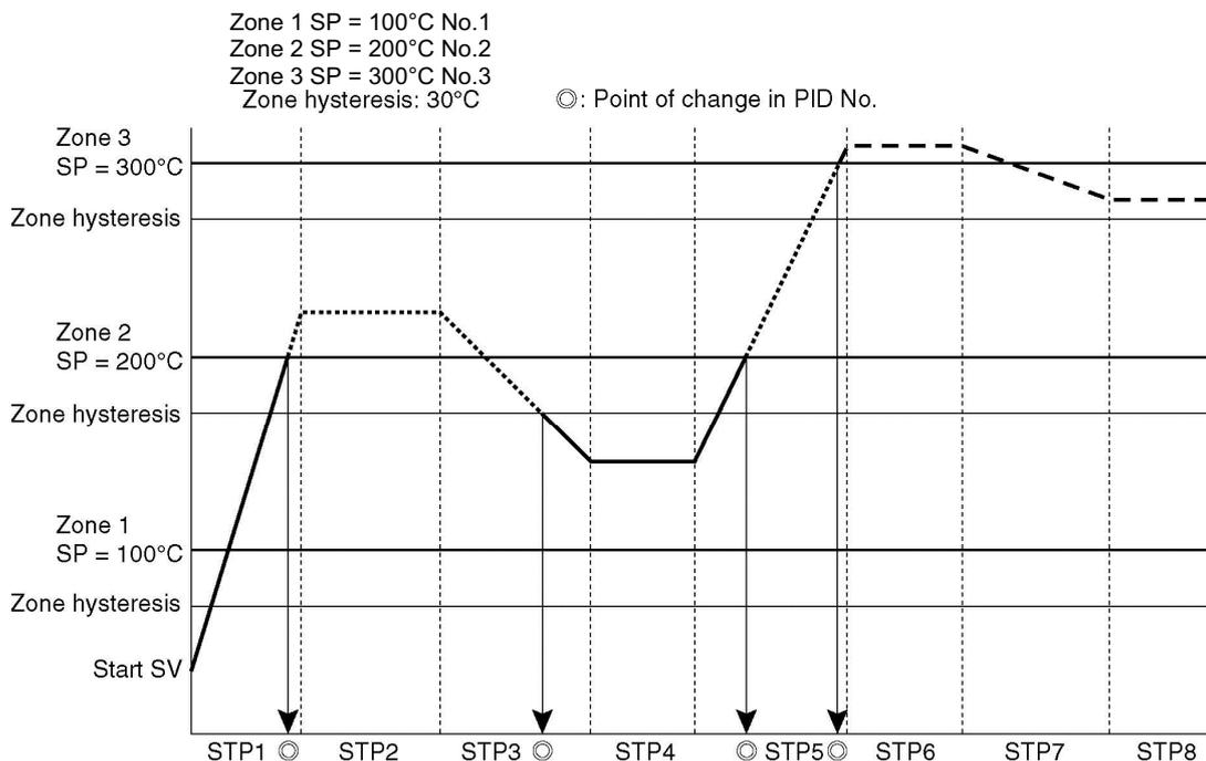
When above diagram shows SV as: Below 200°C → Action with PID No. 1
