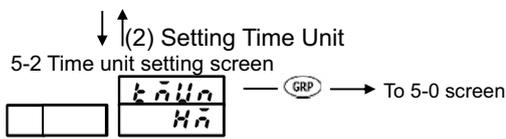
A unit of time used in various items, such as step signal and step time, is set.
